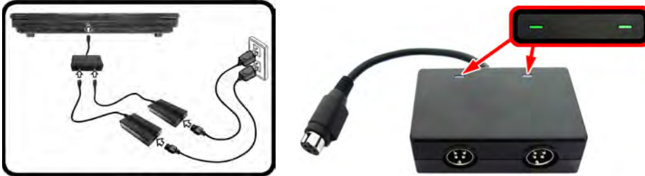
Figure D - 15 - Dual Power Adapters & Converter Box
